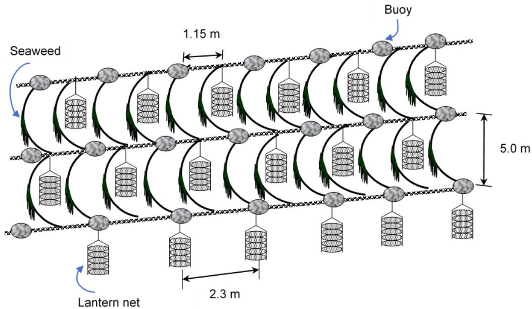
Fig. 3 The structure of longline system for shellfish and seaweed integrated aquaculture
